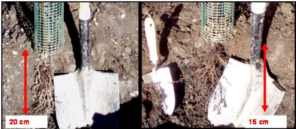
Plate 6: Tree root profiles wide track bulldozer emplaced (left) and narrow track bulldozer emplaced (right)
