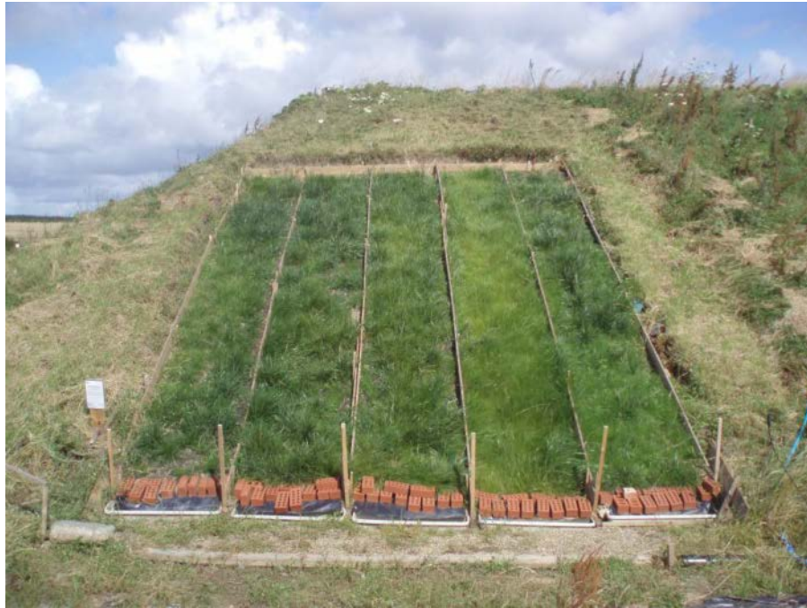
Photo 11. South west block. Treatments left to right: 10 cm incorporated; 5 cm surface; 5 cm incorporated; geotextile.
