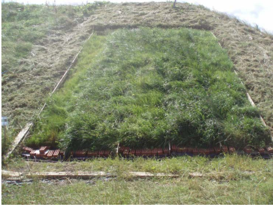
Photo 13: North west block. Treatments left to right: goetextile; 10 cm surface; 5 cm surface; 10 cm incorporated; 5 cm incorporated.
