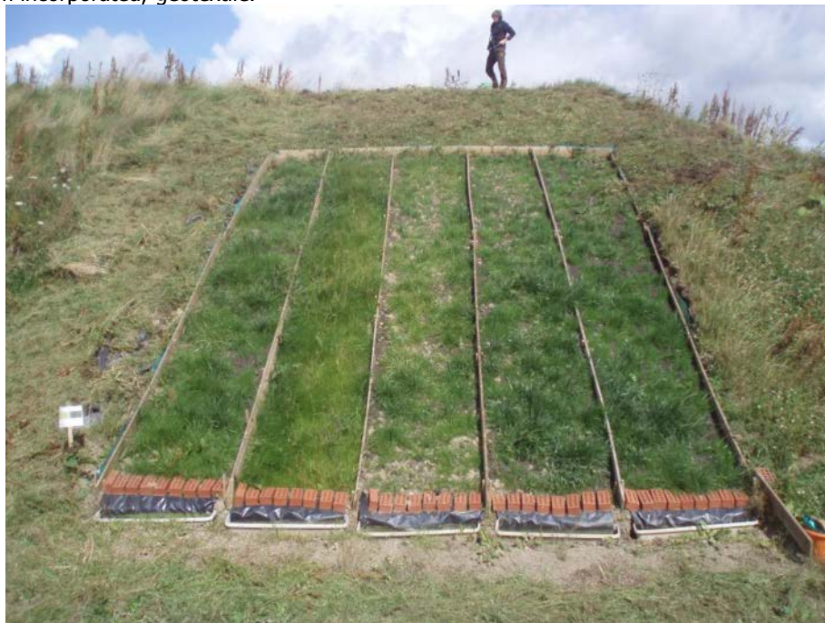
Photo 12: South east block. Treatment left to right: 5 cm surface; geotextile; 5 cm incorporated; 10 cm incorporated; 10 cm surface.
